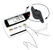
ARotate the Crushing Handle counterclockwise, and fully insert the Sampling Tray into the Testing Chamber. Fully rotate the Crushing Handle until stop is reached, so that the sample may be well crushed. Press the "MEA" (Measure)button, the most reliable moisture content is then displayed to be read directly without using any conversion tables.
